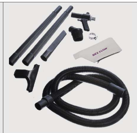
Model 36013 - All Purpose System consists of X-stream™ hand vac plus 10 foot (3 m) vacuum hose with cuffs at both ends, reusable collection bag, cleaning brush, crevice tool, skimmer tool, two extension wands, and stainless steel hose clamp.
